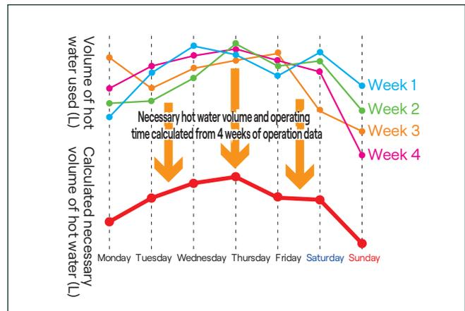
**Energy Saving Function** - This function is an energy-saving function that learns operation patterns from the four previous weeks to prevent unnecessary heating and temperature decreases in stored water through natural heat loss. The use of this function based on operation data stops the unit from boiling water unnecessarily.
